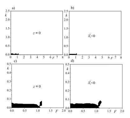
FIG. 2. CS in the network of four coupled VDP oscillators;  $k_1 = k_2 = k$ . (a) Synchronization error *z*, (b) MSF, (c) enlargements of the synchronization error *z*, and (d) MSF. White color: z=0 or  $\lambda_1^T < 0$ ; black color: z > 0 or  $\lambda_1^T > 0$ .
