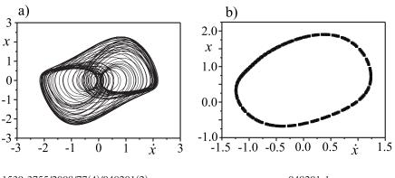
FIG. 1. Quasiperiodic motion of the VDP oscillator: (a) Phase plane and (b) Poincaré section.
